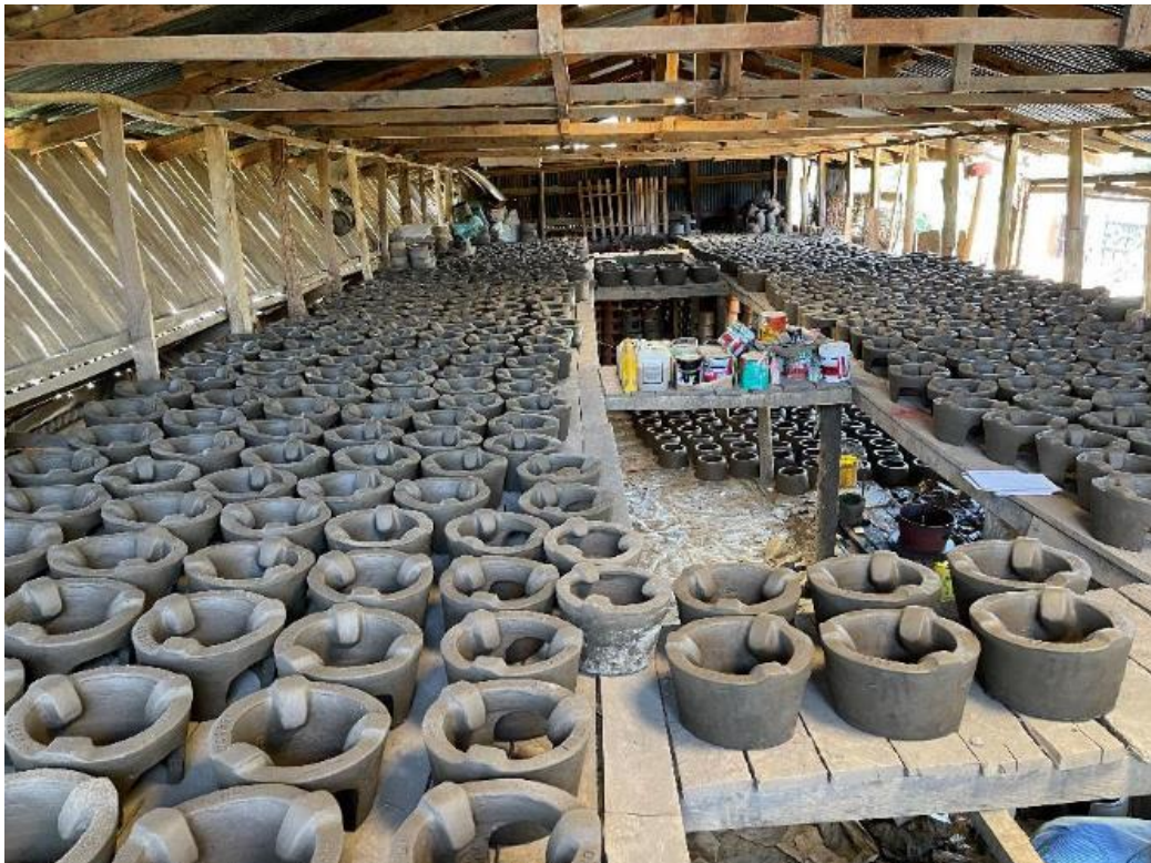
Figure 3. The slow-drying floor for terracotta stove liners at Pauline Cachanja's workshop (FP103)
